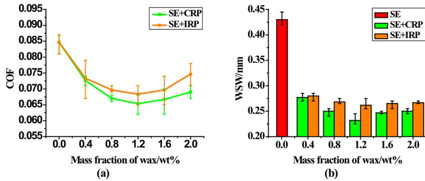
Figure 4 (a) COFs and (b) WSWs of CRP and IRP additives under different load
