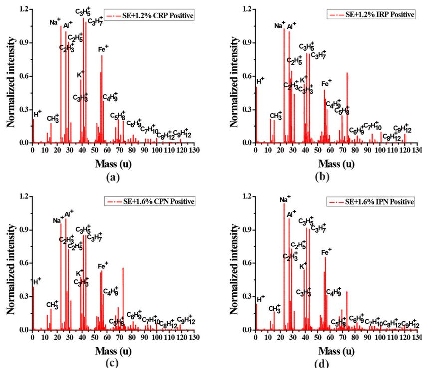
**Figure 9** The negative ions normalized intensity diagrams on worn surfaces lubricated with (a) SE + 1.2 per cent CRP, (b) SE + 1.2 per cent IRP, (c) SE + 1.6 per cent CPN and (d) SE + 1.6 per cent IPN
