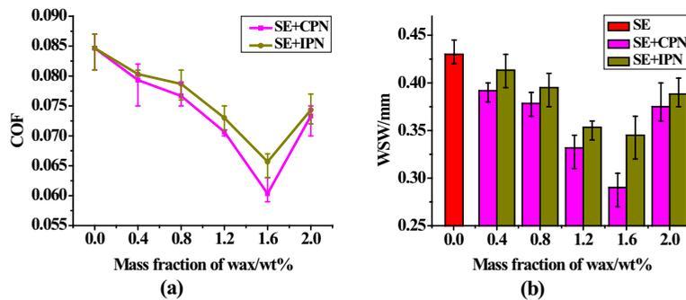
Figure 6 (a) COFs and (b) WSWs of CPN and IPN additives under different load
