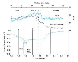
Figure 4. Polarization curve and coefficient of friction (COF) during the sliding test for the NaCl solution in the absence and presence of 0.01 M C8Na under abrasion condition. The vertical solid lines indicate the constant potentials at which sliding wear tests were conducted during following testing.
