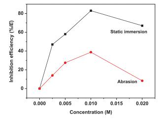
Figure 3. Change of inhibition efficiency of AA5052 in 0.5M NaCl solution containing C8Na with different concentrations under static immersion and abrasion conditions.
