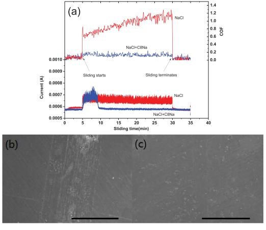
Figure 7. (a) The convolution of current transient and coefficient of friction as function of sliding time before, during and after sliding test at an anodic potential -1.0 V vs Aq/AqCl. SEM image of the wear track produced at -1.0 V vs Aq/AqCl for (b) NaCl solution and (c) NaCl solution containing 0.01 M C8Na. Scale bar: 100 µm.
