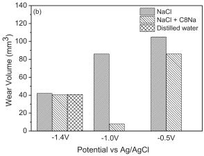
Figure 9. The variation of COF and wear volume at different potential applied for NaCl solution in the absence and presence of 0.01 M C8Na.
