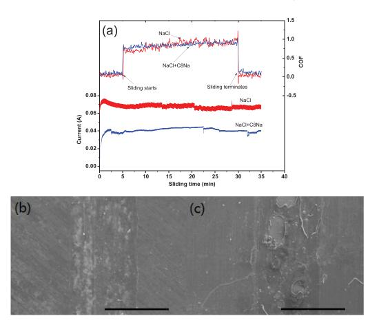
**Figure 8.** (a) The convolution of current transient and coefficient of friction as function of sliding time before, during and after sliding test at -0.5 V vs Ag/AgCl. SEM image of the wear track produced at an anodic potential -0.5 V for NaCl solution in (b) the absence and (c) presence of 0.01 M sodium octanoate. Scale bar:  $100 \mu m$ .
