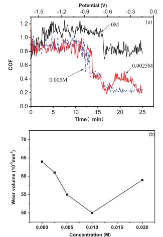
**Figure 5.** (a) The coefficient of friction (COF) during, and (b) wear volume after potentiodynamic test under abrasion condition for NaCl solution in the absence and presence of C8Na with different concentration.
