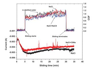
**Figure 6.** The convolution of current transient and coefficient of friction as function of sliding time before, during and after sliding test at a cathodic potential of -1.4 V vs Ag/AgCl.
