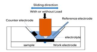
Figure 1. The scheme of the corrosion and tribocorrosion instrument.
