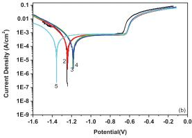
Figure 2. Potentiodynamic polarization curves recorded under (a) static immersion and (b) abrasion conditions in NaCl solution containing (1) 0 M, (2) 0.0025 M, (3) 0.005 M, (4) 0.01 M and (5) 0.02 M sodium octanoate.
