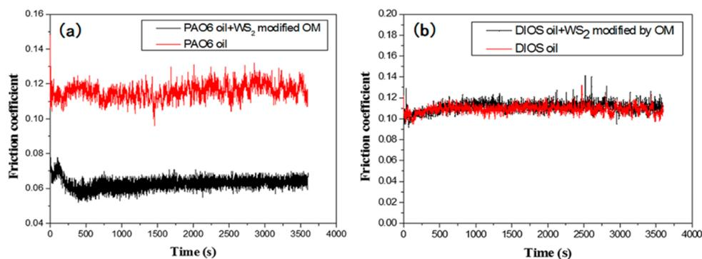
**Figure 1.** Friction coefficient of the steel–steel sliding pair lubricated by (a) PAO6/OM-capped WS<sub>2</sub> and (b) DIOS/OM-capped WS<sub>2</sub> (four-ball tester; load 392 N, speed 1200 rev/min, time 60 min, temperature 75 °C; additive concentration 2.0%).
