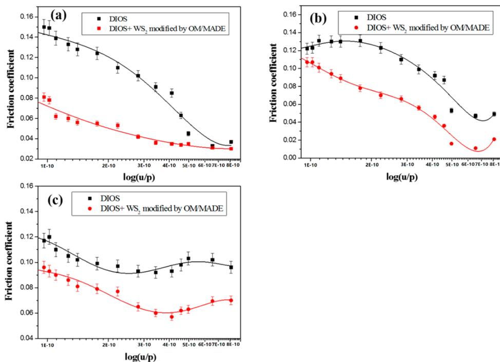
**Figure 6.** Stribeck curves of DIOS oil and DIOS oil with 2.0% of OM/MADE-capped  $WS_2$  nanoparticles at room temperature (a), 75 °C (b), and 150 °C (c).
