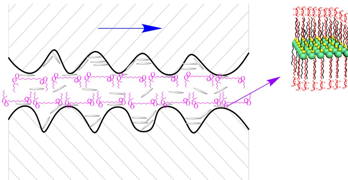
**Figure 10.** Tribological model of OM/MADE-capped WS<sub>2</sub> nanoparticles in DIOS.
