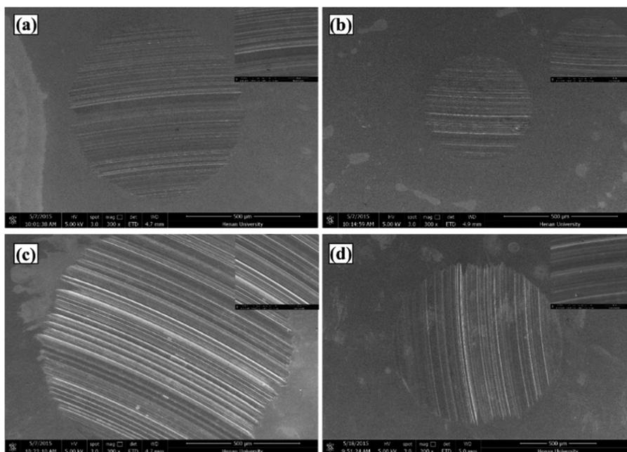
**Figure 7.** SEM images of worn surfaces of steel ball lubricated by DIOS oil (a, 75 °C; c, 150 °C) and DIOS oil with 2.0% of OM/MADE-capped  $WS_2$  nanoparticles (b, 75 °C; d, 150 °C) under different temperatures (DIOS oil was tested at 75 °C).
