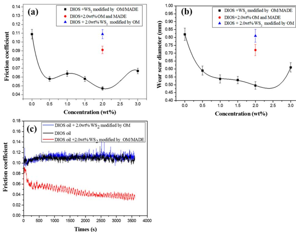
**Figure 4.** Friction coefficient (a) and WSD (b) vs OM/MADE-WS<sub>2</sub> nanoparticles concentration in DIOS as well as friction curves (c) of DIOS, DIOS with 2.0% of OM-capped WS<sub>2</sub>, and DIOS with 2.0% of OM/MADE-capped WS<sub>2</sub> (conditions the same as those in Figure 1).
