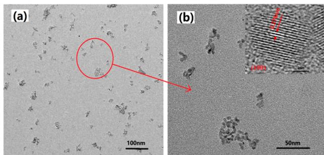
**Figure 3.** TEM (a) and HRTEM (b) images of OM/MADE-capped WS<sub>2</sub> nanoparticles.
