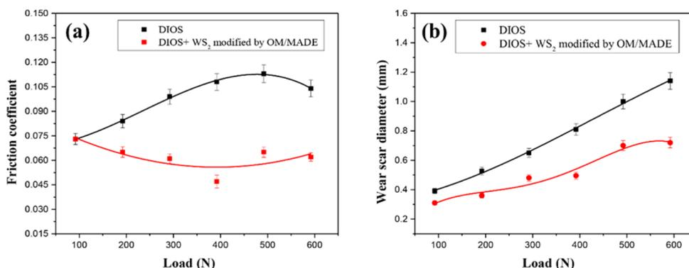
**Figure 5.** Friction coefficient and WSD vs load curves (conditions the same as those in Figure 1 except for load).
