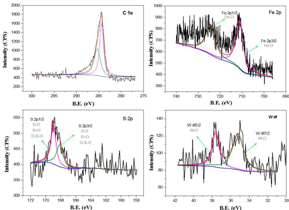
**Figure 9.** XPS spectra of C 1s, W 4f, S 2p, and Fe 2p of worn steel ball surfaces lubricated by DIOS containing OM/MADE-capped WS<sub>2</sub> nanoparticles (conditions the same as those in Figure 8 except for temperature (150 °C); B.E. is the abbreviation of binding energy).
